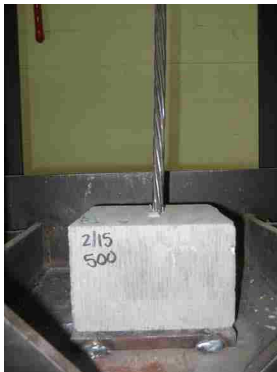
Figure 3.10 Enlarged view of pullout test setup with specimen inside steel cage
