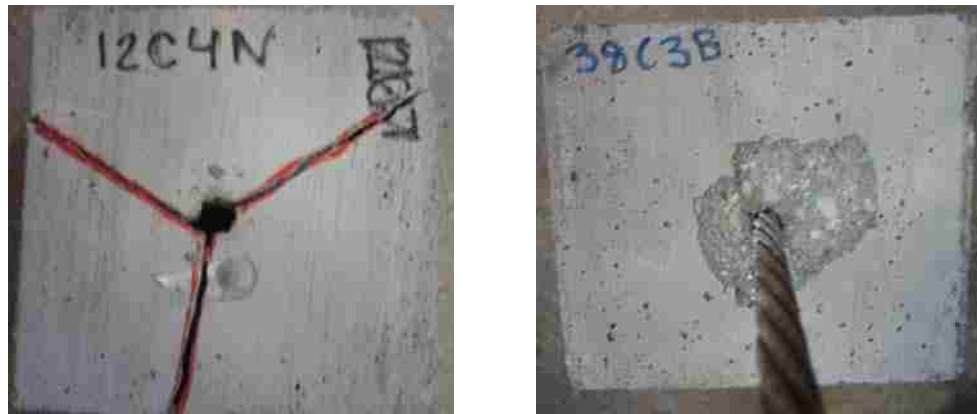
A. left: brittle failure, right: failure taken at 3 in. (76.2 mm) slip
