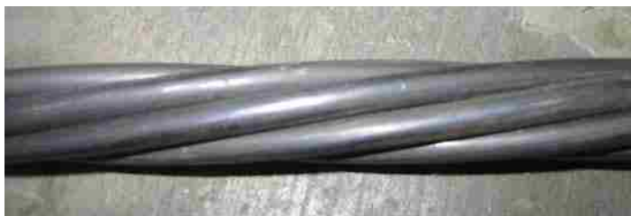
Figure 4.2 Strand exterior after exposure to 800°F (427°C)
