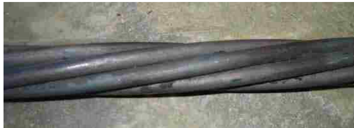
Figure 4.5 Strand exterior after exposure to 1300°F (704°C)
