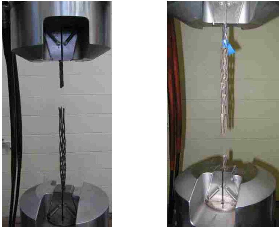
Figure 4.7 Typical failure mode of prestressing strand in tension
