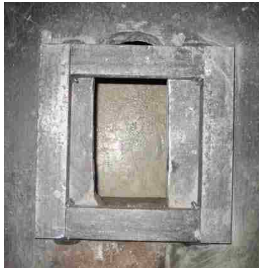
Figure 3.9 Base of pullout cage which concrete block was pulled against
