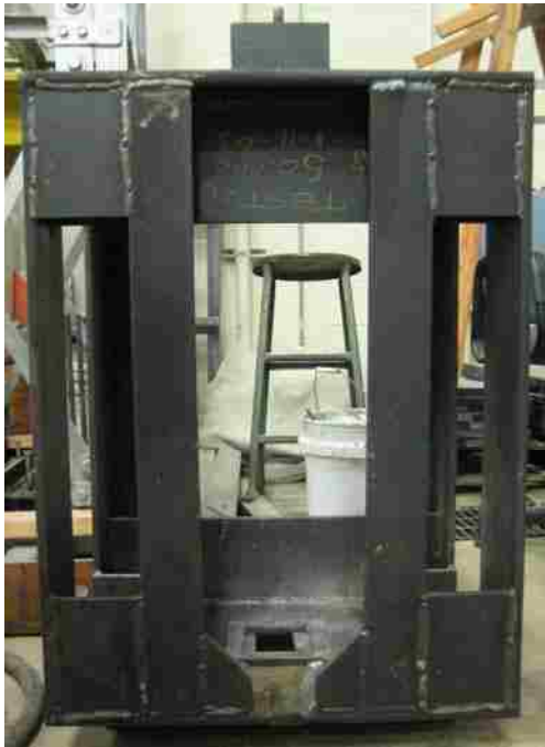
Figure 3.7 Pullout test setup cage prior to testing
