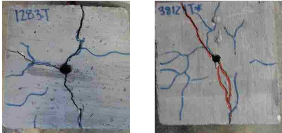
B. left: ductile failure, right: ductile failure
