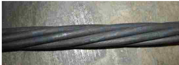
Figure 4.4 Strand exterior after exposure to 1200°F (649°F)
